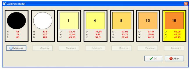
Finish the calibration by clicking on "OK". At this point the successful calibration is confirmed:
