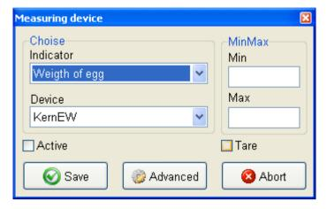
When creating a new device, the indicator (the indicator is what is to be measured) has to be set. Also, the device (the measuring device corresponding to the indicator) has to be selected and set with Min and Max values to be accepted by the program.
